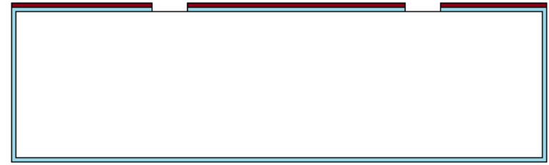
Resist deposition and patterning; SiO2 etching
