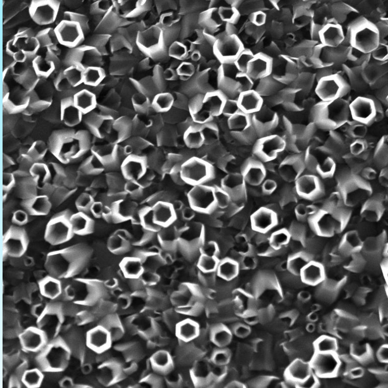
SEM micrograph of CuPc/ZnO(NTs)/ITO structure.
