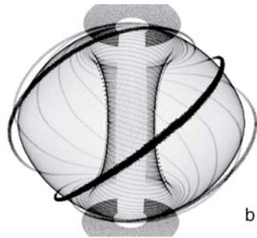
FIG. 4 (color). (a) High-speed video image of the MAST plasma obtained at the start of an ELM. (b) The predicted structure of an ELM in the MAST tokamak plasma geometry, based on the nonlinear ballooning mode theory.
