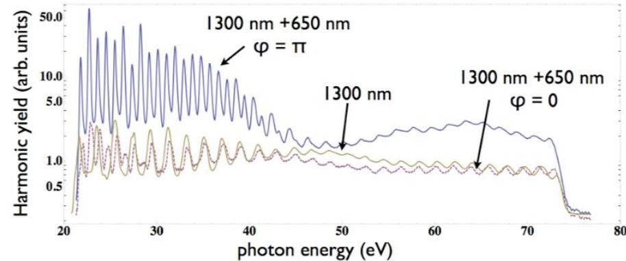
HHG spectra of argon  $\lambda_1=1300$  nm and  $\lambda_2=650$  nm pulses ( $\omega + 2\omega$ ), orthogonal polarisation. **10x HHG enhancement – compensates lower 1300nm efficiency.**
