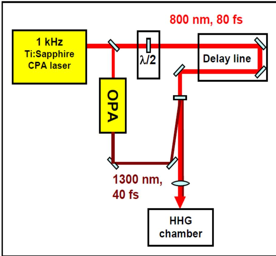
Artemis laser at CLF was used as it has a high power TOPAS synchronised to 800nm used for molecular alignment
