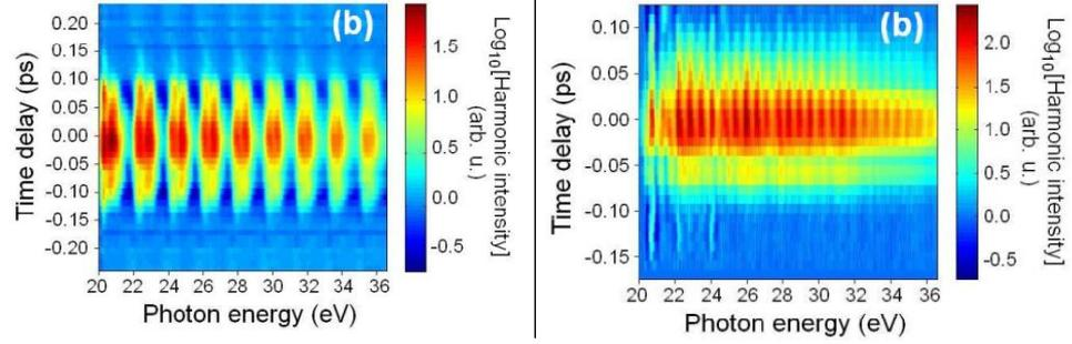
HHG spectra of argon function of delay between  $\lambda_1=1300$  nm and  $\lambda_2=780$  nm pulses, parallel polarisation (normalised 1300 nm HHG).
