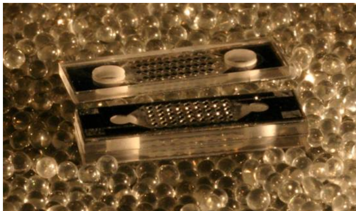
Photo of the fabricated DEP with 3D electric field gradient (asymmetric electrodes)
