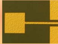
GaN membrane supported FBAR structures before backside etching
