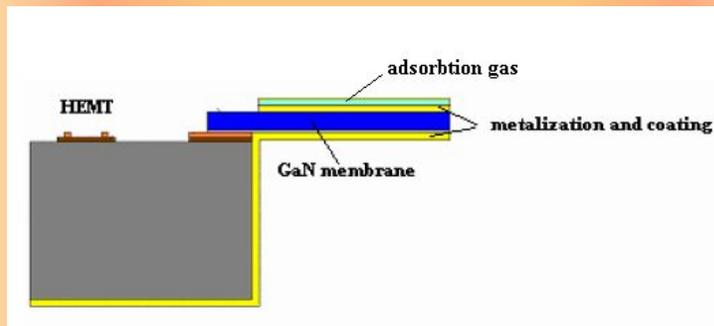
The GaN on silicon structure grown by MOCVD sed for the first FBAR structures ( grown by Azzuro Ltd. Magdeburg)
