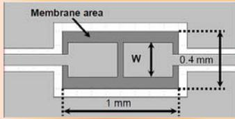
The layout of the AlN FBAR test structure
