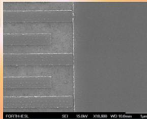
**SEM photo (left) and detail (right) for the 0.5  $\mu\text{m}$  wide finger/ interdigit detector structure manufactured on a 0.78  $\mu\text{m}$  thin GaN membrane**
