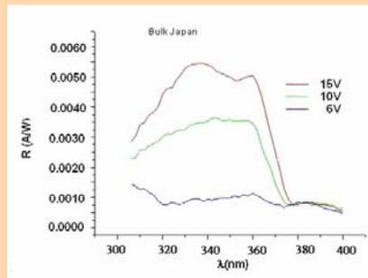
*Responsivity vs wavelength for the 0.5μm finger / interdigit for the UV detector structure- before the silicon substrate removal (thickness of the GaN layer 0.78μm)*
