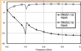
Magnitude of the measures S parameters of the AlN based FBAR  $300\mu\text{m}$  test structure
