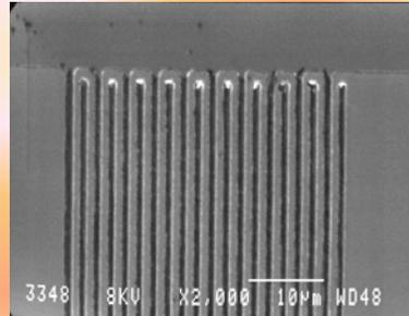
SEM photos of the 1  $\mu\text{m}$  wide Ni/Au (20nm/100nm) lines The interdigit width was also about 1  $\mu\text{m}$
