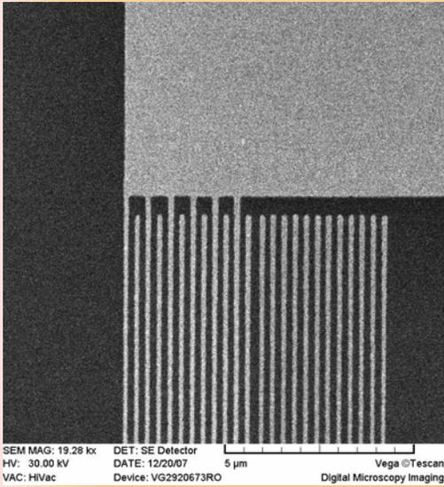
Nanolithography performed at IMT with VEGA 5136 LM SEM from TESCAN and ELPHY Plus Nanolithography equipment from RAITH GmbH
