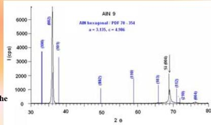
XRD diffraction pattern for a high oriented AlN film sputtered onto Si  $\langle 100 \rangle$  substrate
