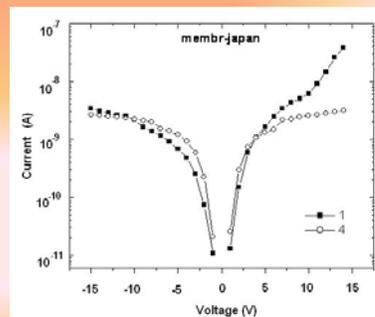
**Dark current for the 0.5  $\mu\text{m}$  finger / interdigit for two UV termed "1" and "4" detector structures- manufactured on 0.78  $\mu\text{m}$  thin GaN membrane**
