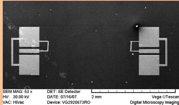
Each IDT structure has 30 digits and 29 inter-digits. The digits and inter-digits have a length of 200 $\mu$ m, and an equal width of 200 nm for one type of test structures and 300nm for the other type.
