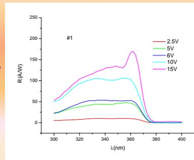
*Responsivity vs wavelength for the 0.5μm finger / interdigit for two UV detector structures- manufactured on 0.78μm thin GaN membrane*
