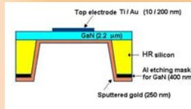
Cross section of the FBAR structure with the evaporated Ti/Au for the top metallization and sputtered Au for the bottom contact. Sputtered Al is used as mask for the bulk-micromachining of the membrane
