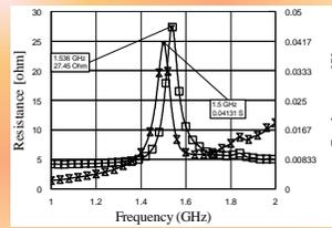
The resistance and the conductance of the two FBARs structures connected in series
