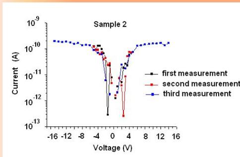
**Dark current for the 0.5  $\mu\text{m}$  finger / interdigit for the UV detector structure-*before* the silicon substrate removal (thickness of the GaN layer 0.78  $\mu\text{m}$ )**
