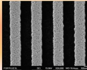
SAW test structure ( $W=300\text{nm}$ )
