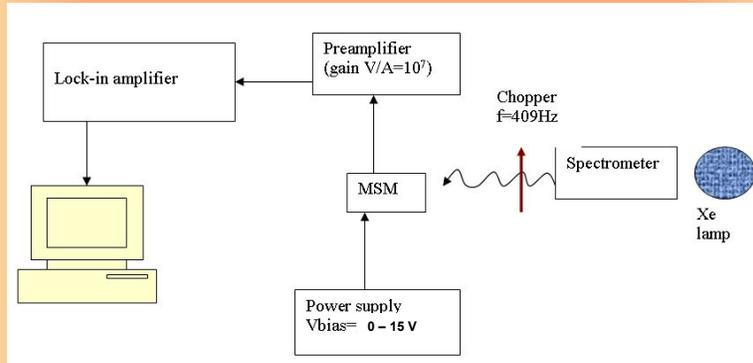
**Optical measurements set-up**
