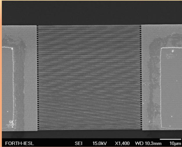
**Series connection of SAWs (detail)**
