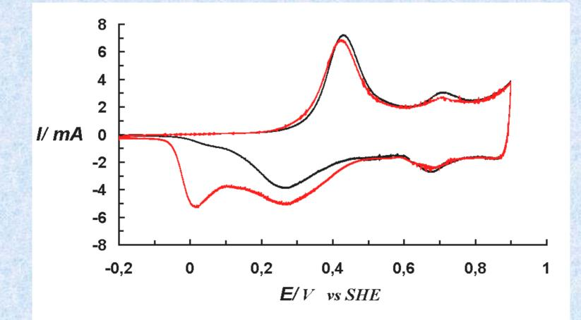
I-t response of CPs electrodes (m=0.6 mg,  $\emptyset 5$ -mm) in oxygen saturated 1M HCl. The electrodes were polarized by stepped  $\Delta E$  from 0.6 to 0.0V
