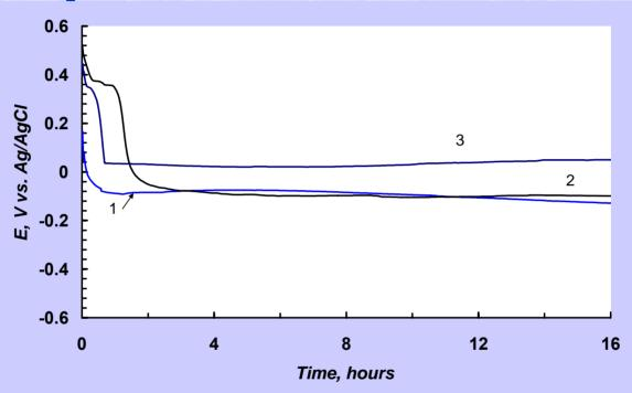
The potential of oxygen electroreduction at the composite *PANI/AMD/PB* electrode is of about 150 mV higher then on other
