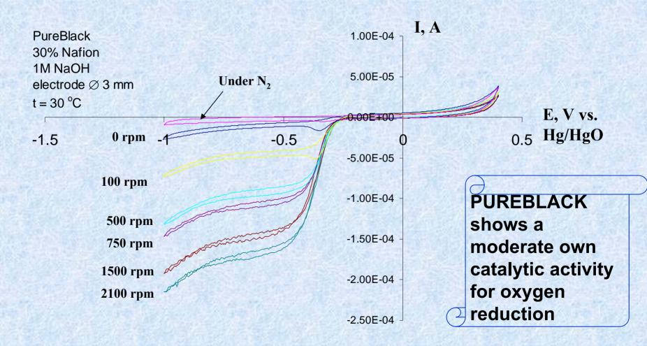
CV of rotating disk electrode based on Pureblack
