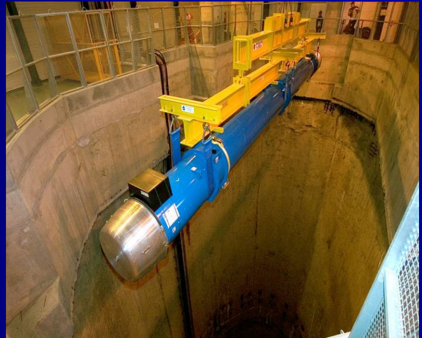
Photo of a transport device in action with a 15m long dipole of 30t
