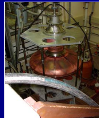
Electrochemical polishing installation
